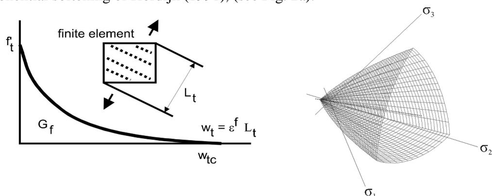
(a) Tensile softening (Hordijk 1991) (b) Three parameter criterion for concrete (Menetrey & Willam (1995))
