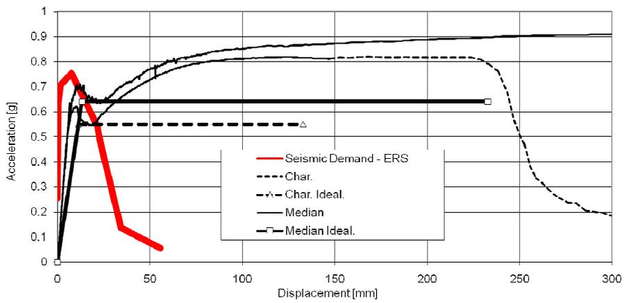
**Fig. 5: Pushover curves based on elastic response spectrum of the local seismic demand.**
