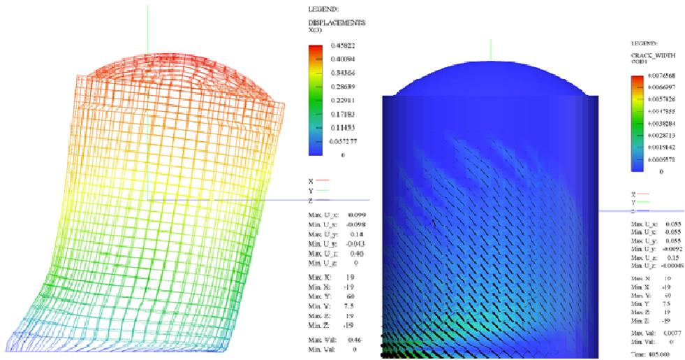
**Fig. 4: Deformed form (left) and crack pattern (right) of the characteristic analysis case.**
