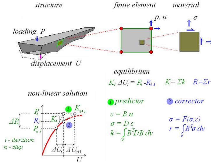
**Fig. 1: Scheme of non-linear finite element analysis**
