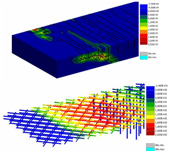
(b) ATENA simulation slab tests,
