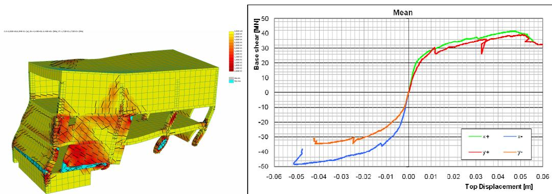
**Fig. 6: Pushover analysis of a reinforced concrete building housing the power plant control room**
